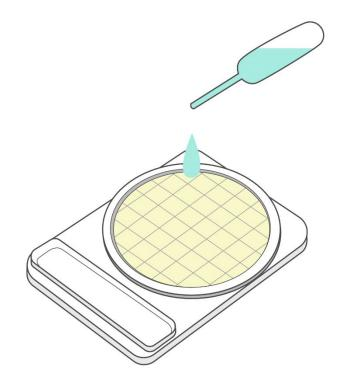
Pipette 1ml of homogenized specimen (to be further diluted if necessary) in the middle of dry sheet of Compact Dry EC.
