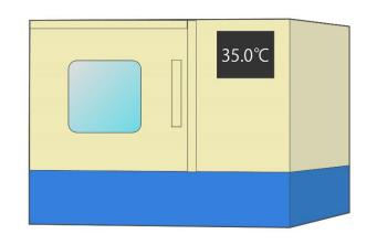
put in an incubator. Incubate 24 hours for EC at 35 +/- 2°C.
