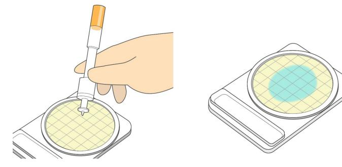
Inoculate 1 ml of wiping solution (to be diluted if necessary), which is obtained from cotton swab,
