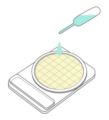
Pipette 1ml of homogenized specimen (to be further diluted if necessary) in the middle of dry sheet of Compact Dry TC.
